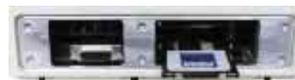
DEA 10 removed cover with D-Sub connector for Floppy Disk and PC-Card memories
