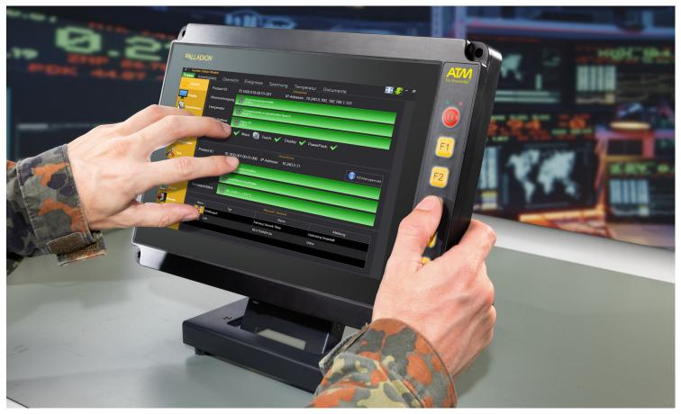
The capacitive multi-touch display of the PALLADION panel PC features full HD resolution and high luminance and is also readable with night vision devices.
