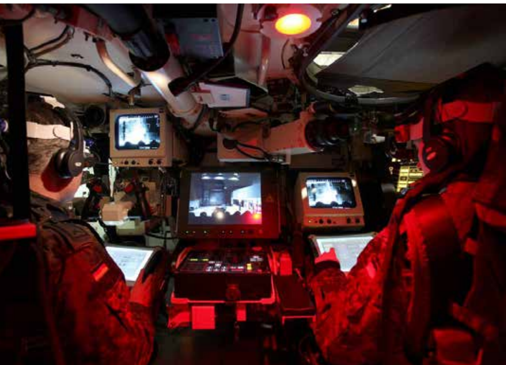
Central user interface in connection to other AIFV Puma control devices
